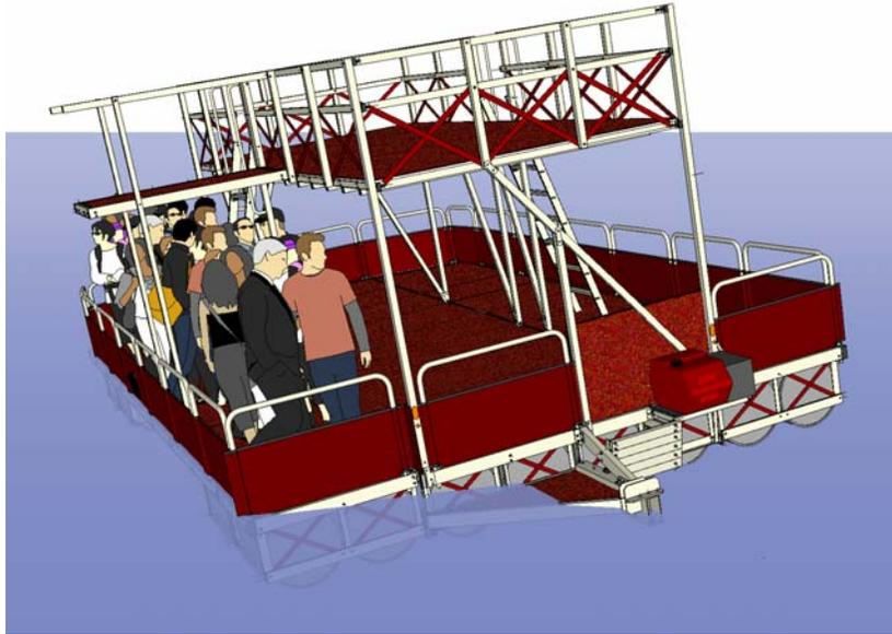
Figure 3 – All Passengers on Lower Level to Port Side
